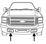
equipped with a gasoline engine have the plug exposed on the driver side of the vehicle; vehicles equipped with a Diesel engine have the plug exposed on the passenger side of the vehicle.
